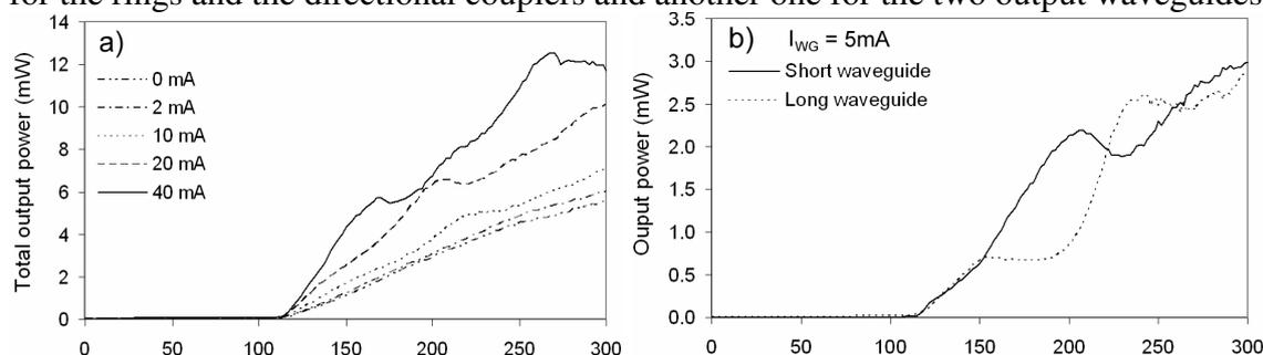
Figure 4: a) Total optical output power as a function of  $I_{\text{Ring}}$  for different  $I_{\text{WG}}$ . b) Short and long output waveguides power as a function of  $I_{\text{Ring}}$  for  $I_{\text{WG}} = 5\text{ mA}$ . The output powers are corrected for coupling and optical isolator losses.  $T = 12^\circ\text{C}$ . The directional coupler gap is 1.2  $\mu\text{m}$ .
