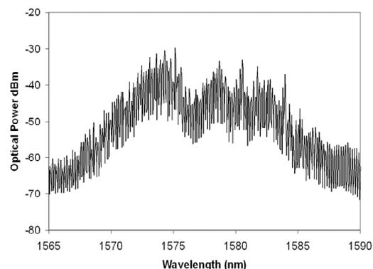
Figure. 2. Lasing spectrum of the deeply etched FP QD laser for  $I = 300 \text{ mA}$  and  $T = 12^\circ\text{C}$ , (resolution 0.1 nm).
