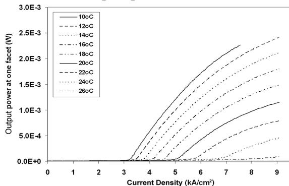
Figure 1: Output power at one facet of the deeply etched FP QD laser as a function of current density for different temperatures. The light was collected using an objective lens ( $\text{NA} = 0.65$ ).
