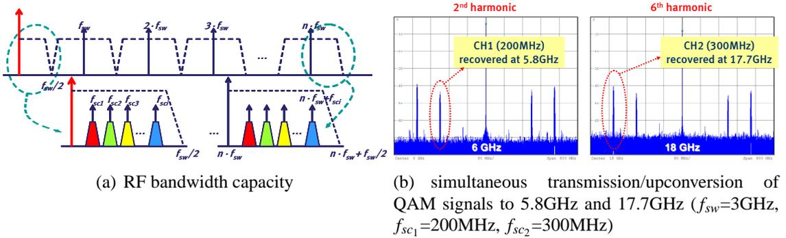
Figure 2: RF bandwidth capacity and multistandard support
