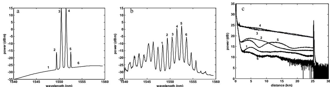
Fig 2 (a) Input spectrum, (b) output spectrum, (c) distribution of the power of channels 1-6
