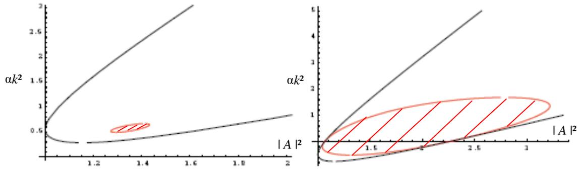
**Fig. 2: Marginal stability of the mean-field equation. The open curves correspond to the original equation [Eq. (1)], whereas the closed curves are for the equation with the real bilaplacian term [Eq. (6)]. The detuning is taken equal to  $\Delta = 1.45$  (left graph) and  $\Delta = 2.5$  (right graph). Unstable regions are hatched.**
