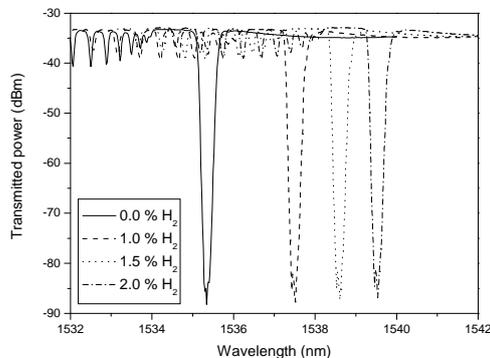
Fig. 1. Transmitted spectrum of a 4 cm long FBG in response to different  $H_2$  concentrations in dry air at ambient temperature.
