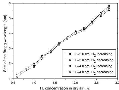
Fig. 2. Shift of the Bragg wavelength as a function of the  $H_2$  concentration in dry air at ambient temperature for two grating lengths.
