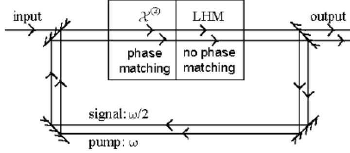
**Fig. 1:** A degenerate optical parametric oscillator in which a crystal with  $\chi^{(2)}$  nonlinearity converts energy from a pump beam to a signal beam. The left-handed material (LHM) modifies the linear propagation properties of the signal beam.
