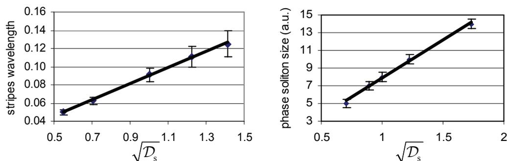
**Fig. 3:** Scaling of the typical size of dissipative structures with the signal diffraction coefficient.
