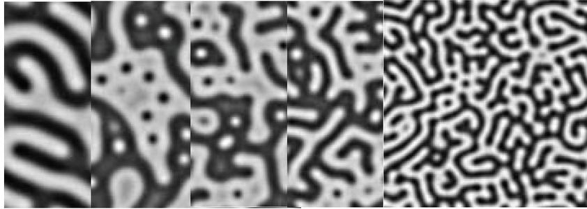
**Fig. 4: Phase domains/solitons emerging from the output mirror above the lasing threshold. Signal diffraction strength is decreased from left to right. Pump diffraction is constant.**
