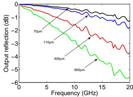
Figure 4: Output reflection coefficient vs. frequency for several photodetectors at  $-5$  V bias voltage.
