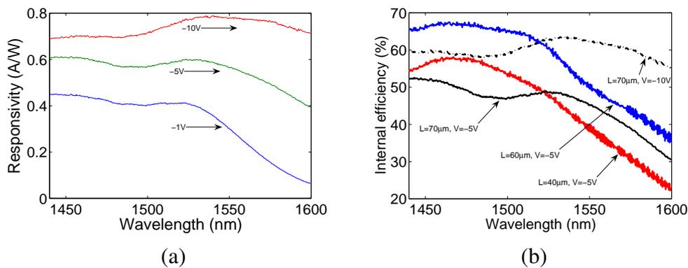
Figure 3: (a) Internal responsivity as a function of wavelength for a  $70\mu\text{m}$  long photodetector at bias voltages of  $-10$ ,  $-5$ , and  $-1$  volts. (b) Internal efficiency as a function of wavelength for several WGPDS and bias voltages.
