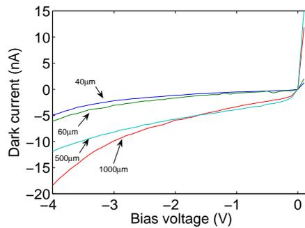
Figure 2: Dark I-V curves for several photodetectors.
