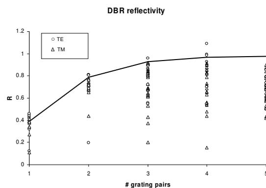
Figure 7: Measured DBR reflectivity
