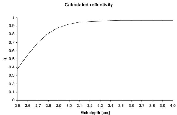
Figure 4: Calculated reflectivity of a 3-period DBR grating in air
