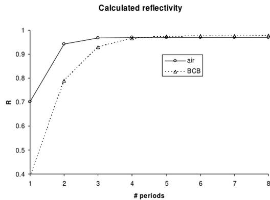
Figure 2: Calculated grating reflectivity for gratings in air (solid line) and BCB (dashed line)
