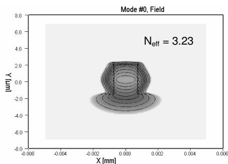
Figure 3: Logarithmic presentation of the field in a 3.5  $\mu\text{m}$  deep etched waveguide
