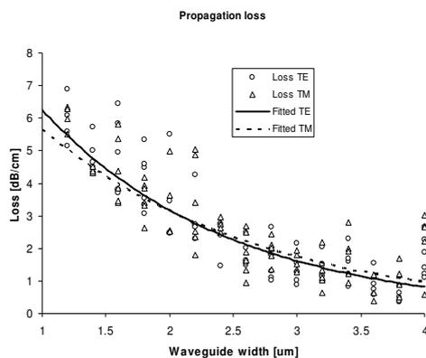
Figure 6: Measured propagation losses
