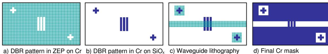
Figure 5: Lithography process. First, the DBRs are written by e-beam lithography (a), then the DBR pattern is etched into the chromium mask (b), then the waveguides are defined by optical lithography (c), and are also etched into the chromium mask (d).
