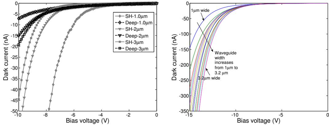
Figure 2: (left) Measured dark currents for deeply etched and shallowly etched phase shifters for different waveguide width. (right) Measured dark currents for deeply etched phase shifter dark currents for different waveguide width.
