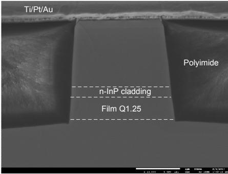
Figure 1: SEM image of a  $2 \mu\text{m}$  wide deeply etched waveguide phase shifter.
