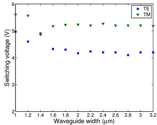
Figure 4: Average switching voltage of five identical 2 mm long deeply etched phase shifters at each width.
