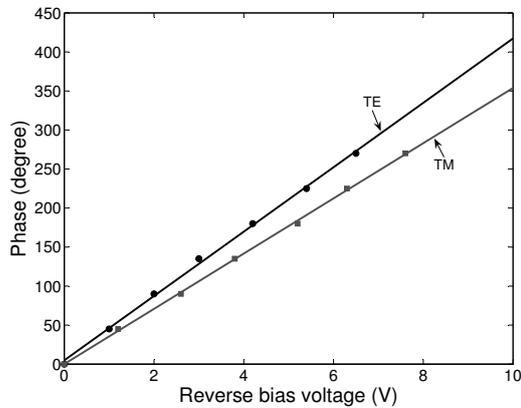
Figure 3: Phase shift as a function of the reversely biased voltage for 2 μm wide, 2 mm long deeply etched waveguide phase shifter.
