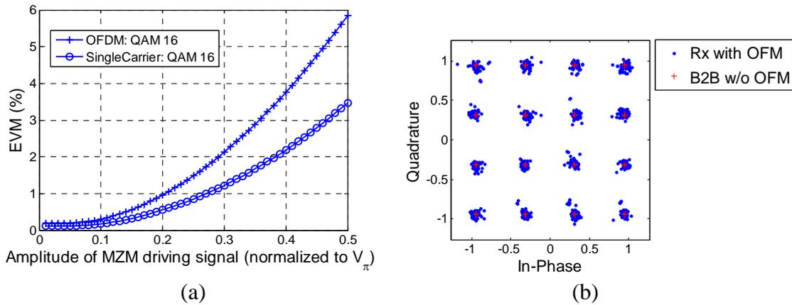
Fig. 2. (a) Error vector magnitude (EVM) value as a function of driving signal amplitude, for OFDM and single-carrier 16-QAM signals. (b) Comparison of constellation of transmitted and received OFDM signal when the amplitude of driving signal is  $0.5 V_\pi$ .
