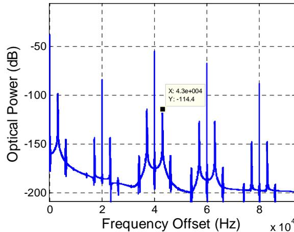
Fig. 3. Optical power spectrum of the output signal from transmitter in an OFM RoF down-link, with sweep frequency and 16-QAM sub-carrier frequency equal to 20 KHz and 3 KHz respectively, and the data tip labels (x, y) = (4.3e4 Hz, -114.4 dBm).
