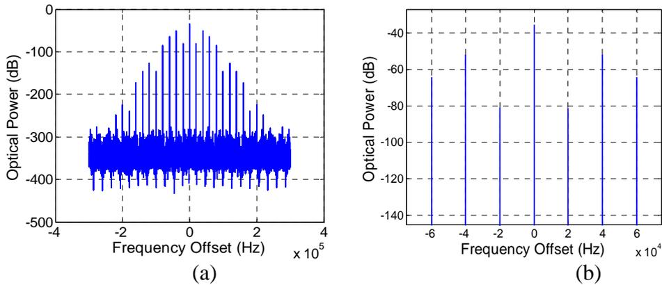
Fig. 2. Optical power spectrum of the output signal from MZI, frequency is offset from central frequency of the laser diode. (b) is a zoomed view of (a). The sweep frequency  $f_{sweep}$  is 20 KHz.
