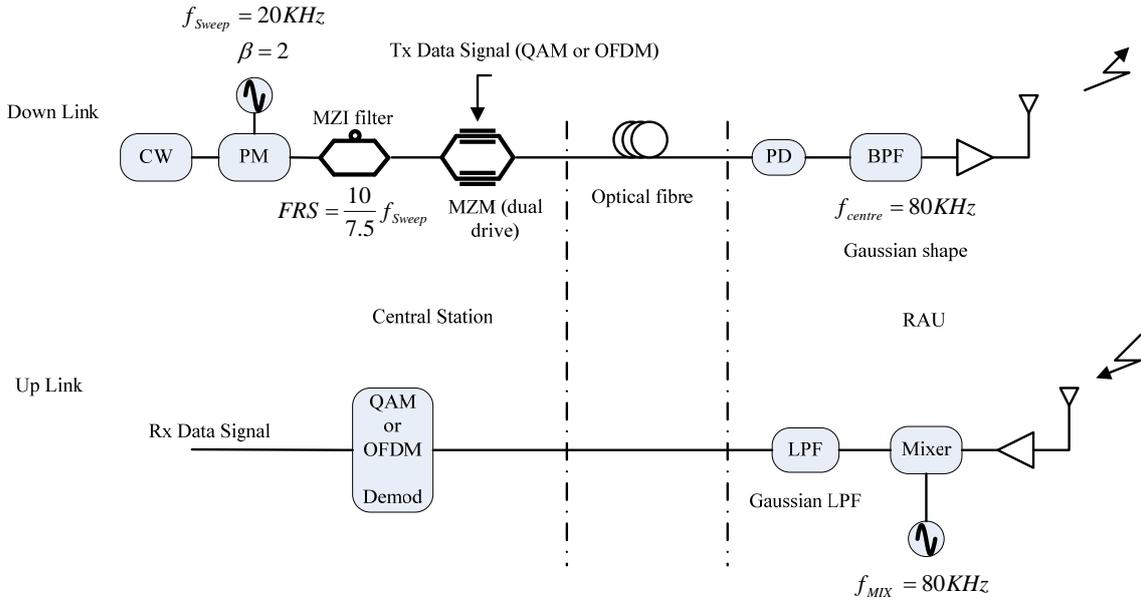
Fig. 1. Illustration of OFDM infrastructure for RoF system. CW: continuous wave, PM: phase modulator, IM: intensity modulator, MZI: Mach-Zehnder interferometer, PD: photo-detector.
