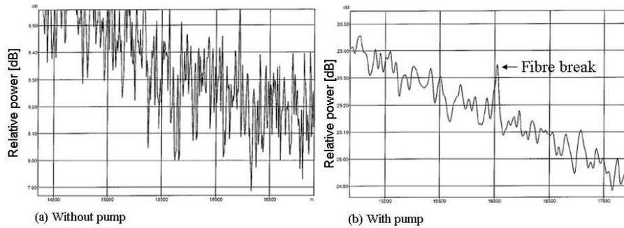
Figure 4: Zoom of the OTDR trace signal around the fibre break (located at 16 km) and using a span of about 200 m: (a) without pump, (b) with pump.
