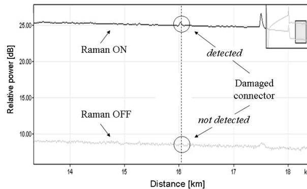
Figure 5: Zoom of the OTDR signal around the damaged FC/PC connector (16 km) and with a span of about 5 km.
