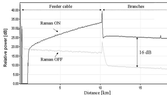
Figure 3: OTDR trace with and without activation of the pump.
