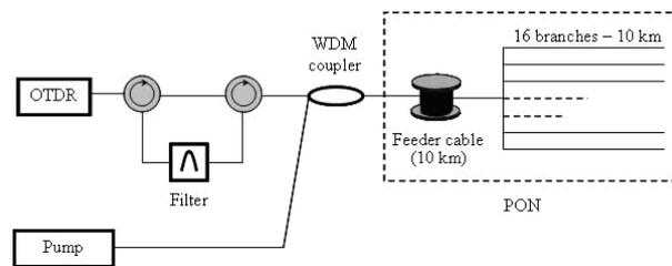
Figure 1: Principle of dynamics enhancement.
