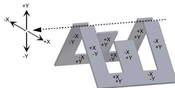
Fig. 4 The displacement of the fiber tip +X, -X, +Y, and -Y as function of the heated positions of the tuning frame.
