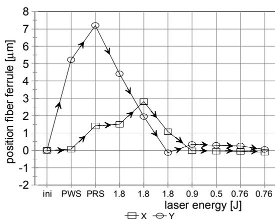
Fig. 6. Pigtail process executed at a prototype micro-system. The shifts as a result of PWS and PRS are fully compensated.
