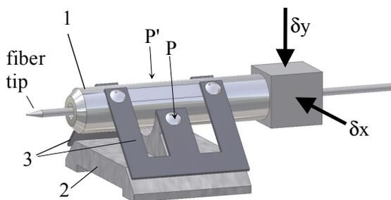
Fig. 3 Schematic presentation of the fiber support micro-system. (1) fiber ferrule including fiber, (2) solid sub-support, and (3) two tuning frames to fine-tune the fiber tip around the pivot point, which is created by points (P) and (P').
