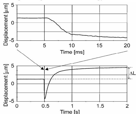
Fig. 2 Measured dynamic response of a metal sheet, which is sketched in figure 1. Upper graph: first expansion of 5  $\mu\text{m}$  is measured during the laser pulse duration of 5 ms. During the cooling down period (lower graph), shrinkage in the metal sheet is measured which results in a net displacement  $\Delta L$  of 3  $\mu\text{m}$ .
