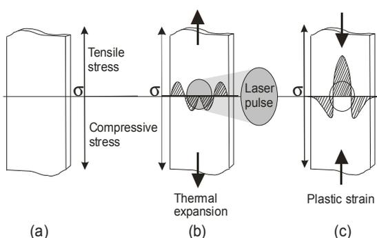
Fig. 1. Principle of laser contraction: (a) the initial stress ( $\sigma$ ) in a metal sheet is assumed to be zero. (b) Heating up the metal beam locally. Thermal expansion occurs, resulting in plastic deformation. The stress in the center becomes compressive. (c) Contraction arises from the plastic deformation of the metal sheet after the heated zone has been cooled to room temperature. The nature of the stress in the center is tensile, generating plastic strain.
