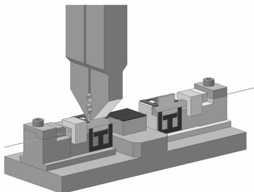
Fig. 7. An artist's impression of the implementation of two micro-systems in one device needed for an optical in- and output fiber.
