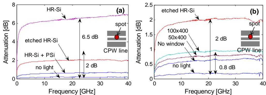
Fig. 4. Photo-Induced attenuation for different substrate types (a) and for different etched window sizes,  $L \times W$  in  $\mu\text{m}$  (b).
