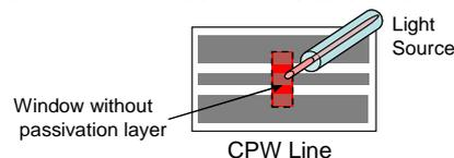
Fig. 3. New design of photo-induced switch on HR-Si with a trap-rich passivation layer.
