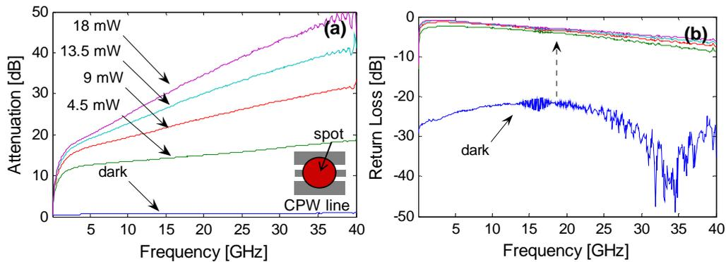
Fig. 1. Photo-induced attenuation (a) and return loss (b) of the optical RF switch on HR-Si under various effective illumination power levels.
