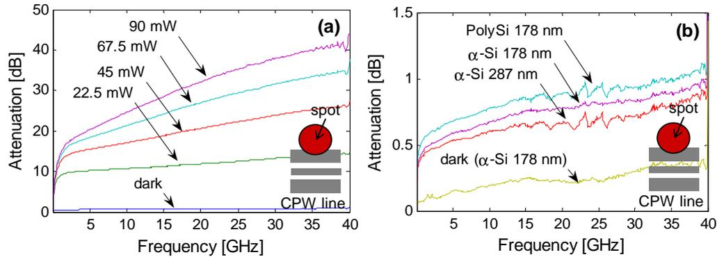
Fig. 2. Attenuation due to optical crosstalk for a CPW line on HR-Si (a) and on HR-Si with different passivation layers for 90 mW of effective optical power (b).
