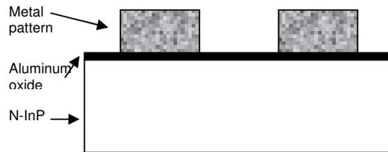
Figure 1: Cross-sectional view of the layers.
