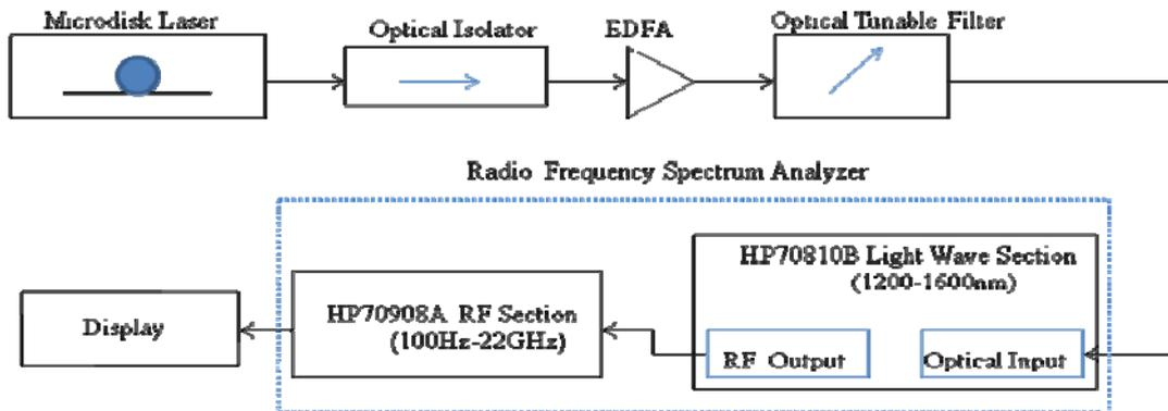
Figure 2. Experimental set-up for beat frequency measurements
