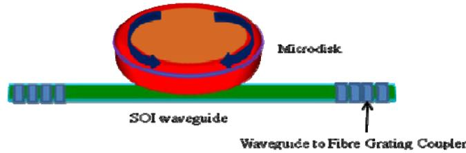
Figure 1. Schematic of a microdisk laser
