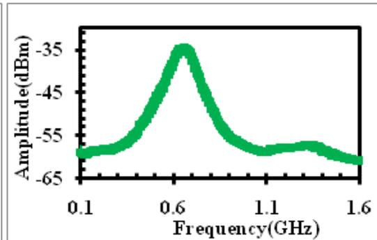
Figure 4. RF Spectrum for MD2 at 2.5mA
