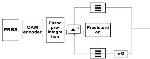
Figure 1 QAM transmitter
