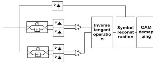
Figure 4 QAM receiver
