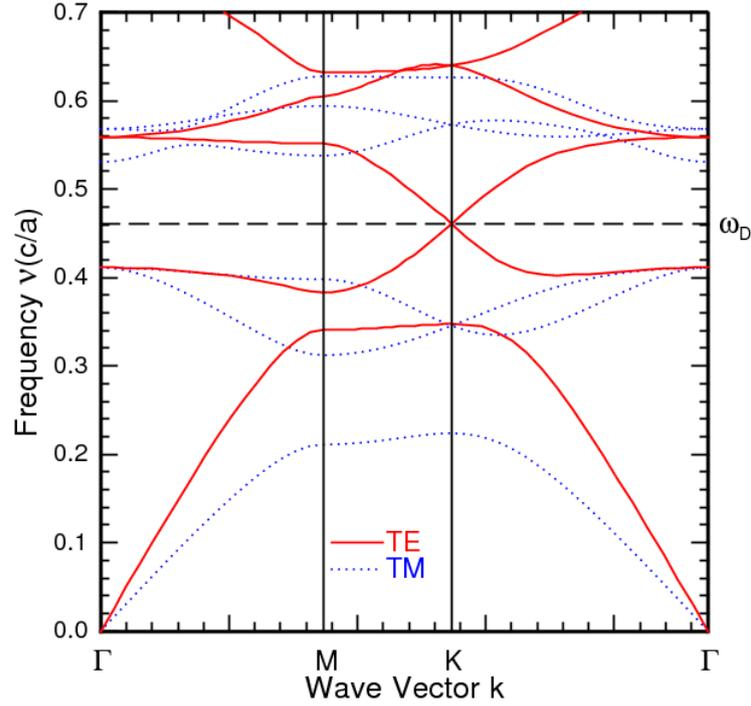
Figure 1: Calculated photonic bandstructure for a triangular lattice of pillars with a dielectric constant  $\epsilon = 12$ . The bandstructure for TE polarization (solid lines) shows an isolated Dirac point at the K-point for a normalized frequency of 0.461, indicated by the horizontal dashed line.
