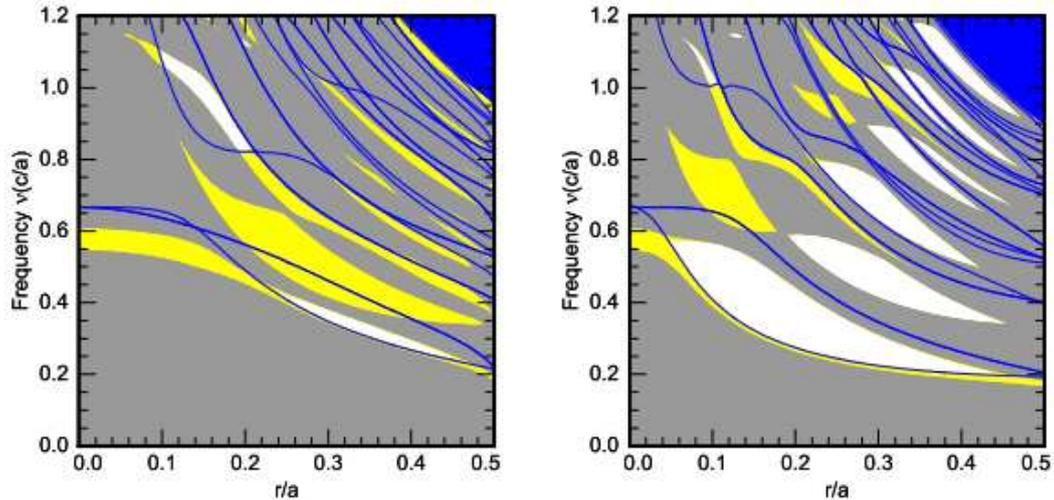
Figure 2: Dirac map of a photonic crystal structure consisting of a triangular lattice of pillars with a dielectric constant  $\epsilon = 12$  for TE polarization (left) and TM polarization (right). The colors indicate the existence of a mode in the  $\Gamma M$  direction (grey area) or the  $\Gamma K$  direction (yellow area). The blue lines correspond to the frequencies of the bands calculated at the K-point. Isolated Dirac points are found whenever these lines are inside a yellow region.
