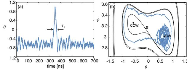
Figure 1: Numerical solutions of Eqs. (1)-(2) revealing a single excitable pulse in time domain (a) and its projection on the phase space (b). The parameters are the following:  $\delta = 4.5\%$ ,  $\phi_K = 1.5$ . (a)  $J = 0.659$ , (b)  $J = 0.691$ .
