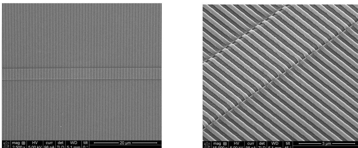
Figure 2: SEM images of the Bragg gratings in the  $\text{SiO}_2$  cladding on top of an  $\text{Al}_2\text{O}_3:\text{Er}^{3+}$  waveguide
