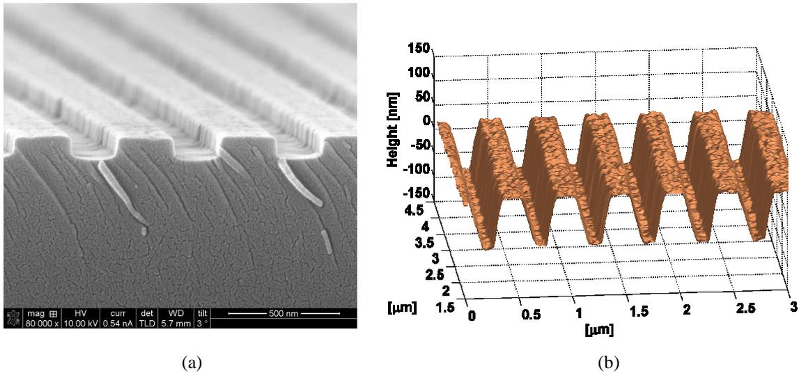
Figure 3: (a) SEM cross-sectional image of a Bragg grating in the  $\text{SiO}_2$  cladding;
