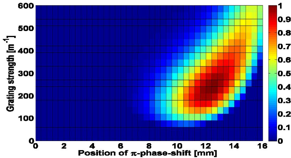
Figure 1: Normalised laser output power as a function of grating strength and phase-shift position
