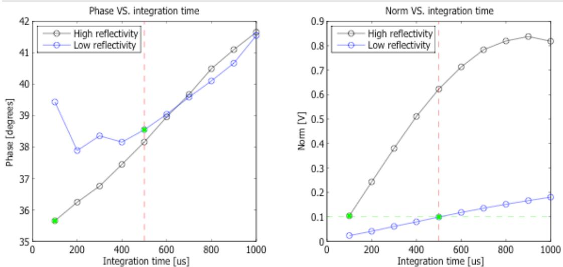
Fig 4 Measured distance (left) and norm (right) vs. integration time for high- and low-reflectivity targets averaged over 1000 measurement cycles
