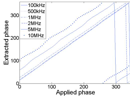
Fig 2 Measured versus applied phase shift of an optical signal [2].
