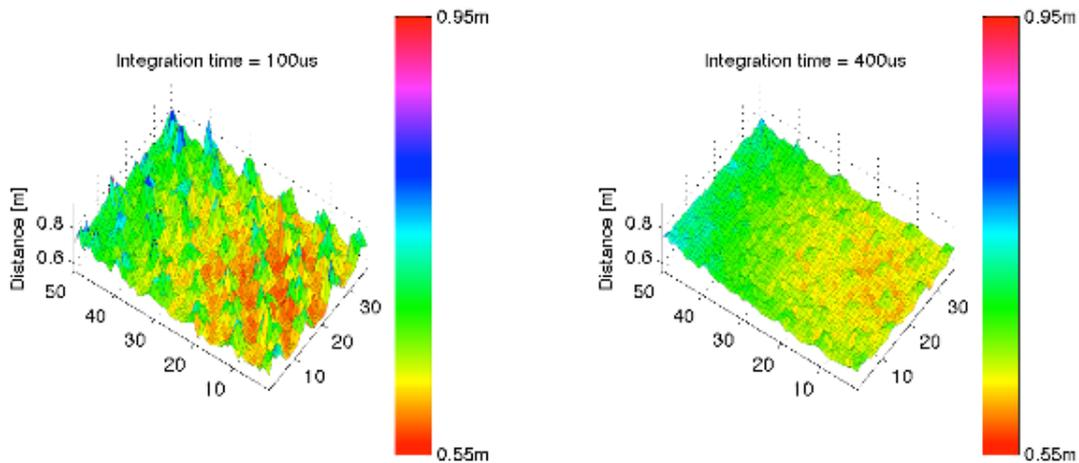
Fig 3 Depth map of the checkerboard pattern for integration times of 100µs (left) and 400µs (right)
