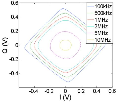
Fig 1 I-Q plot of a CAPD device. For low frequencies, the plot is diamond-shaped. For higher frequencies, the plot converges to a circle [2].
