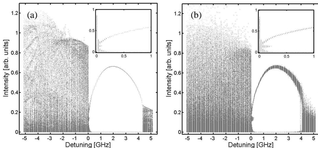
**Fig. 3.** Extrema of the laser intensity with respect to frequency shift. Spontaneous emission noise is neglected in (a) and taken into account in (b). Insets are enlarged views in the range  $\delta = 0$  to 1 GHz.
