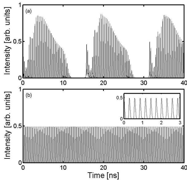
**Fig. 2.** Time trace of the output of the laser subject to optical feedback without frequency shift (a) and with an adequate frequency shift  $\delta = 400$  MHz (b).
