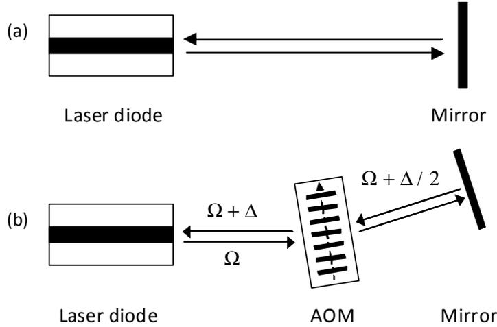
**Fig. 1.** Schematics of a laser diode subject to a conventional optical feedback (a) and to a frequency-shifted optical feedback (b).
