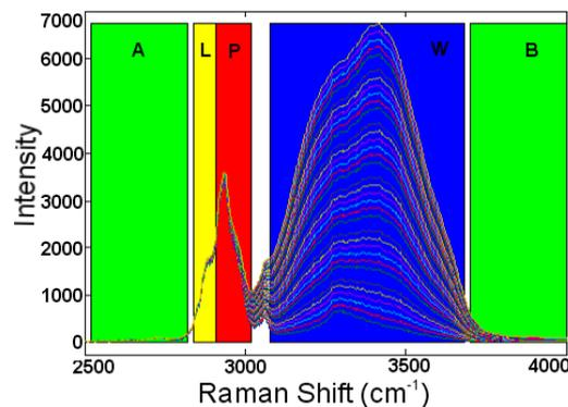
**Fig. 1.** Raman spectrum of the skin for different values of water concentration, with bands A and B used to correct for background variations, L is the lipid band, P the protein band and W the water band.
