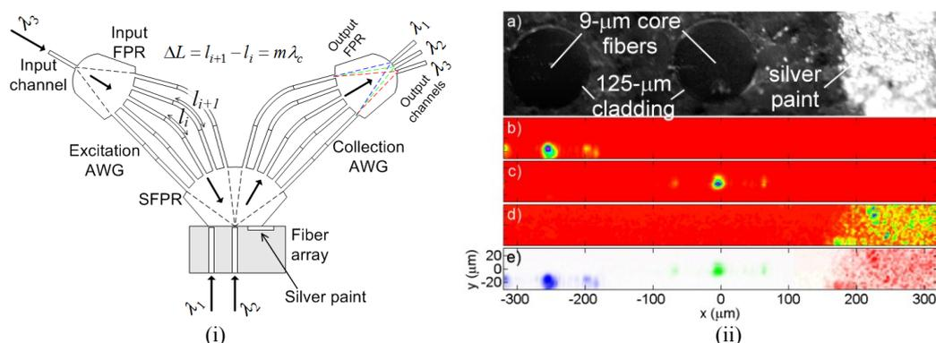
**Fig. 3.** Confocal arrangement of two arrayed waveguide gratings (i); (ii-a) 9  $\mu\text{m}$  fiber array used as a sample; (ii-b,c,d) measurement from output channels centered at 831, 841, and 856 nm; (ii-e) resulting multiwavelength image.
