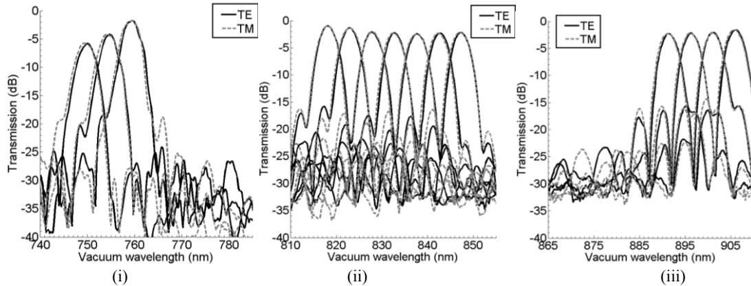
**Fig. 2.** Response of AWG in the wavelength range from 740 nm to 910 nm, for both TE and TM polarizations: (ii) central channels; (i,iii) outer channels.
