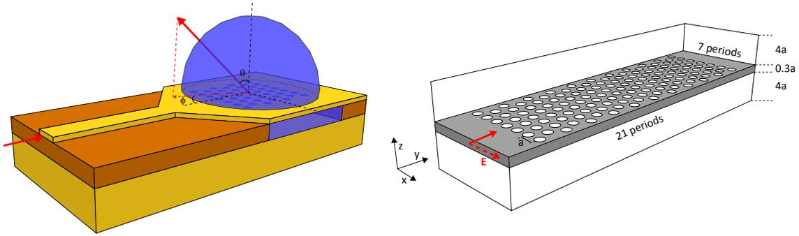
Figure 1: Light enters the PhC biosensor through a waveguide and is coupled to free space as a beam with inclination  $\theta$  and azimuth  $\phi$  (left). The simulated structure used for FDTD simulations is shown in the right figure. All sizes are normalized to the lattice constant  $a$ .
