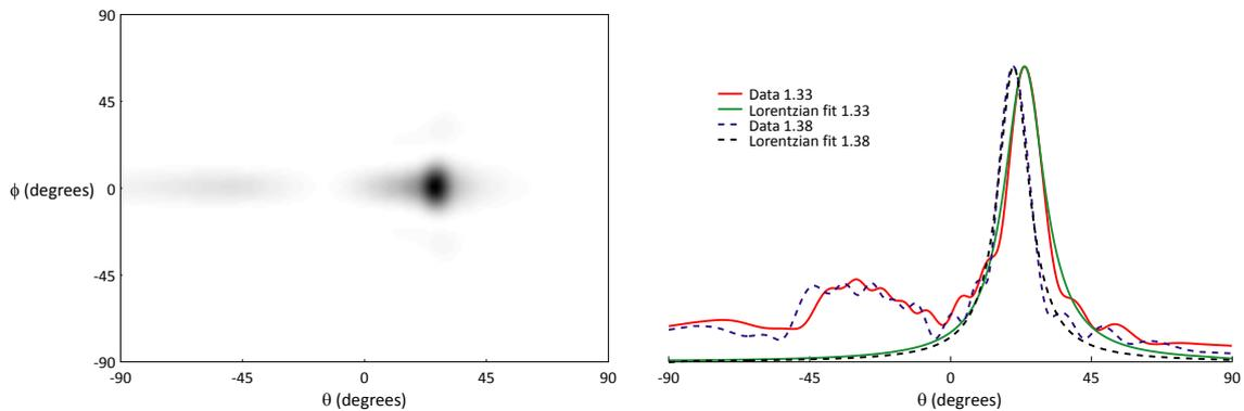
Figure 2: The angular spectrum (left) and cross-section at  $\phi=0^\circ$  (right) of the vertically projected Poynting vector of the proposed structure with a symmetric cladding (i.e. refractive index above and below PhC slab equals that of the holes) at normalized frequency 0.53488. A Lorentzian resonance shape is clearly visible.
