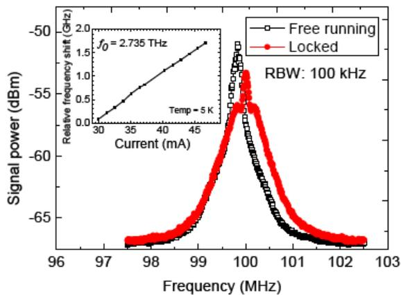
FIG. 2. (Color online). A typical power spectrum of the beat signal of the THz QCL that is phase locked to a microwave reference recorded by the spectrum analyser with a low resolution bandwidth (RBW) of 100 KHz. For comparison, a spectrum of the free-running QCL is also shown. The inset shows a relative frequency shift of the free-running QCL versus the biasing current at 5 K. The starting frequency is 2.735 THz.
