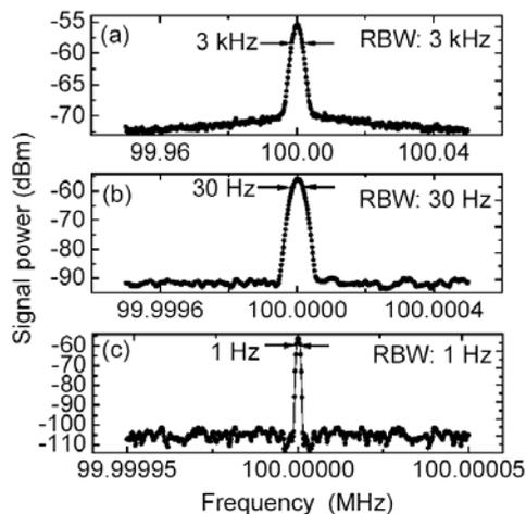
FIG. 3 Power spectra of the beat signal of the THz QCL that is phase locked to a microwave reference recorded by the spectrum analyser with different resolution bandwidths (RBW) and spans, but a fixed video bandwidth (VBW) of 300 Hz. A 3-dB linewidth of the beat signal is also indicated. To avoid confusion, we note that this linewidth is not the actual linewidth of the QCL (see text)
