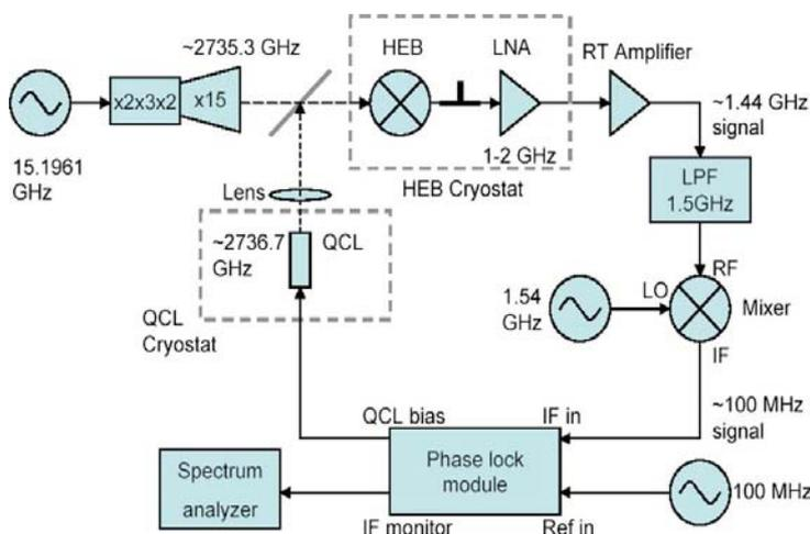
Fig. 1 Schematic diagram of the experimental setup to phase lock a THz QCL at 2.7 THz to a microwave reference.
