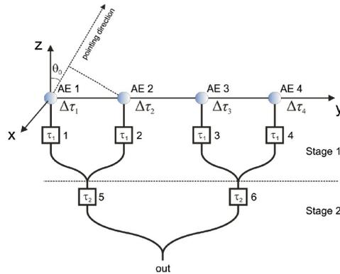
Figure 1. Architecture of a symmetric binary tree  $4 \times 1$  OBFN feeding a 4-elements linear array. Note how delay units 5 and 6 are shared among multiple paths.
