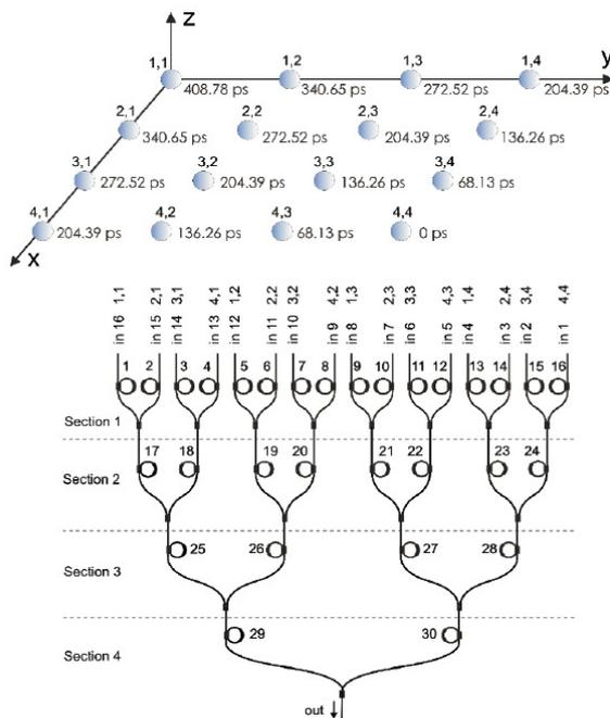
Figure 3. Ex. of OBFN for a 4x4 Ku-band planar antenna.
