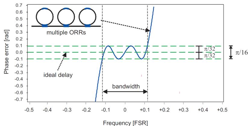
Figure 2. ORR-based delay elements: phase error response
