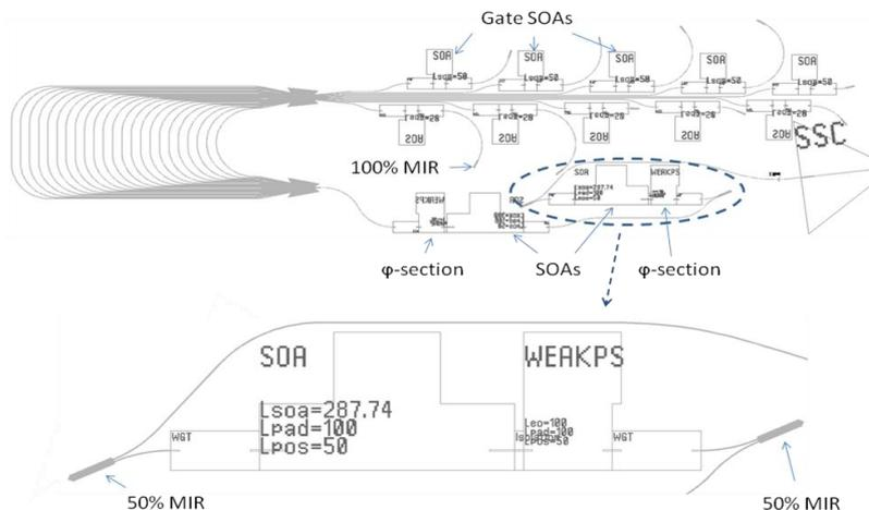
Figure 5: Mask layout of tunable laser chip (top) with detail of FP-laser part (bottom). The chip is constructed using Basic Building Blocks such as SOAs, phase shifters (WEAKPS), spot size converter (SSC) and waveguide transition elements (WGT). The circuit size is roughly 1 x 4 mm.
