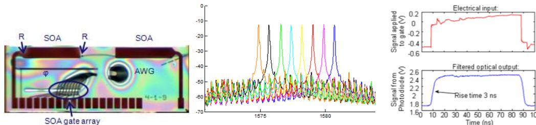
Figure 3: Picture of previously realized tunable laser (left) (chip size: 1.0 x 2.5 mm, no intra-cavity phase shifter present in this device), detail of laser spectrum (middle) and measured switching behavior (right)
