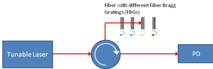
Figure 1: FBG readout using a tunable laser as light source
