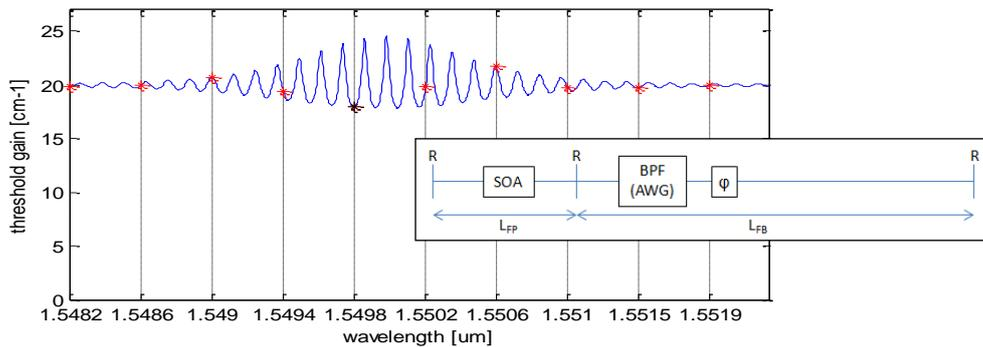
Figure 4: Calculated threshold gain for  $L_{FP}=822 \mu\text{m}$  (50 GHz mode spacing) and  $L_{FB}=2671.5 \mu\text{m}$  and a 200 GHz AWG Band Pass Filter (BPF). The vertical dashed lines indicate the FP laser mode positions. The stars show the intersections between the laser modes and the feedback resonances. The star with the lowest threshold gain shows which mode will start lasing.
