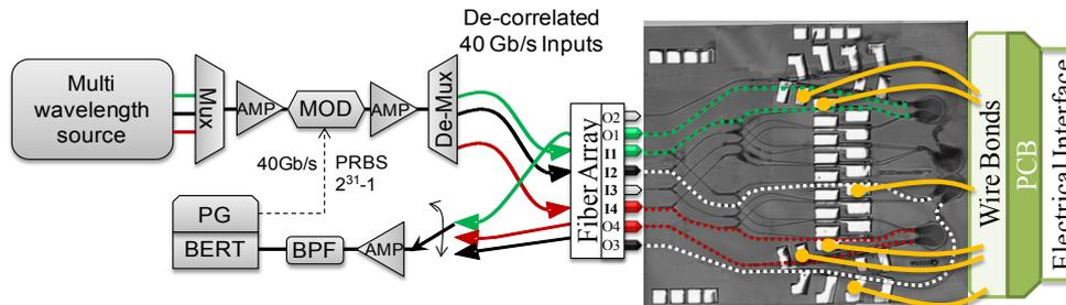
Fig 3. Experimental setup for simultaneous multi-path routing of 3x40 Gb/s data channels
