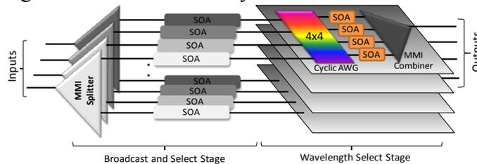
Fig. 1 Schematic of the 4x4 broadcast and select cross-connect.
