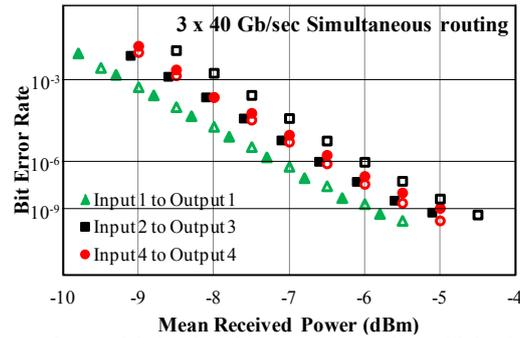
Fig 4. Bit error rate assessment for multiple simultaneous routed 40 Gb/s channels. Back-to-back data for each channel is shown with open symbols.
