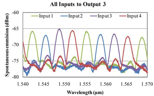
Fig 2. Overlaid spectral response of the cyclic AWG
