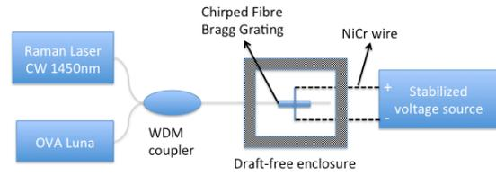
Figure 2 : Sketch of the experimental setup used to control and measure the group delay variation.
