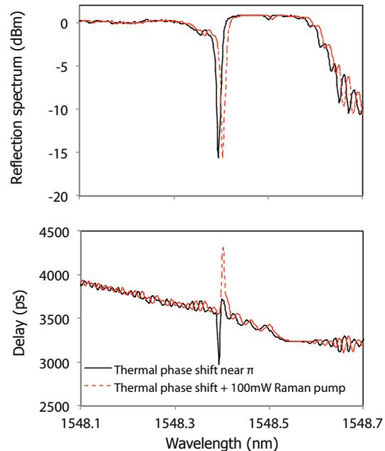
Figure 4 : Switch between negative and positive delay variation using 100 mW Raman pump.
