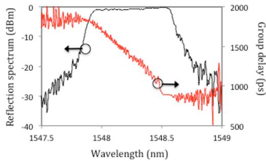
Figure 1: CFBG reflected spectrum and associated group delay evolution (light launched through the long-wavelength port).
