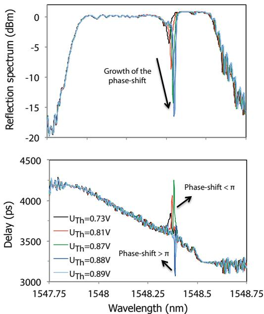
Figure 3 : CFBG reflected spectrum and group delay evolution for different thermally-induced phase shift values
