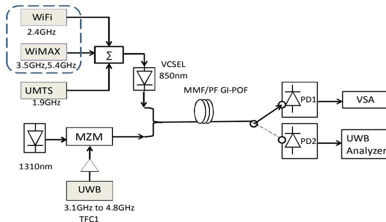
Fig. 2 Experimental setup
