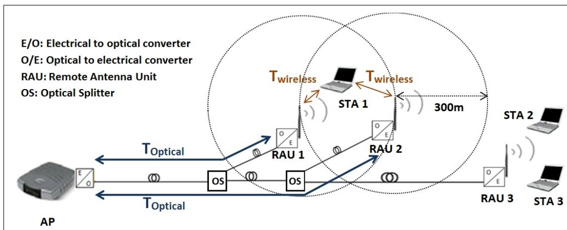
**Figure 1:** Illustration of an IEEE 802.11 wireless access network using the radio-over-fiber technology
