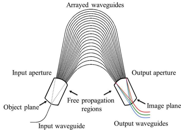
Fig. 1. Schematic layout of an arrayed waveguide grating (AWG).
