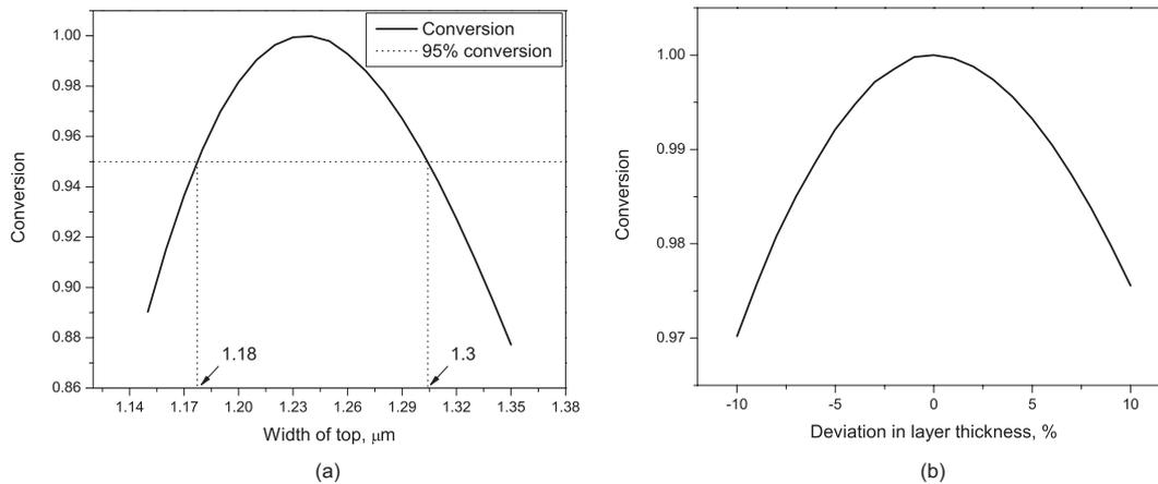
Figure 2: (a) Conversion of converter as function of width of top. Dotted horizontal line shows conversion limit of 95 %. (b) Conversion as a function of deviation in layer thicknesses of converter's stack.
