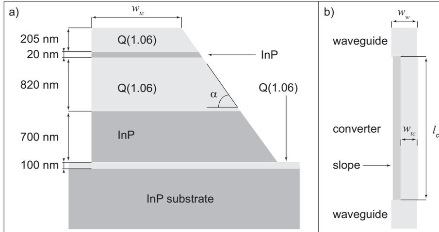
Figure 1: (a) Cross section of converter used to calculate modes of converter. (b) Top view on converter.  $w_{tc}$ , width of top; Q(1.06),  $\text{In}_{0.87}\text{Ga}_{0.13}\text{As}_{0.27}\text{P}_{0.73}$  used as guiding layer;  $w_w$ , width of input and output waveguides;  $\alpha = 55^\circ$ , angle of sloping sidewall made by  $\text{Br}_2\text{-CH}_3\text{OH}$  wet etching .
