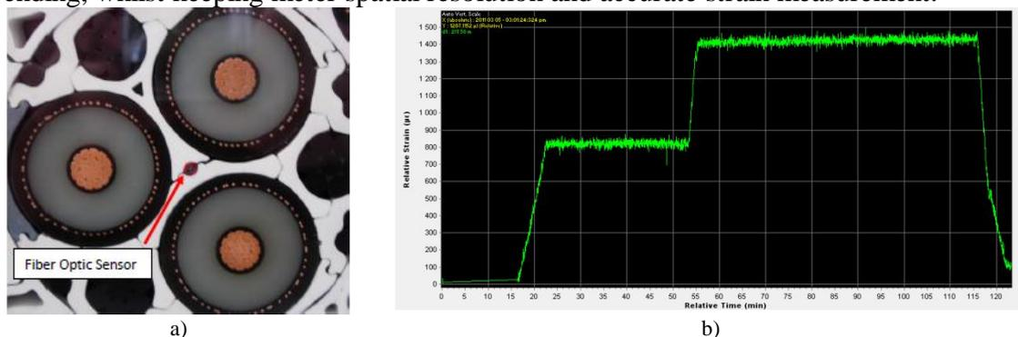
Figure 1. a) Sensor integrated in the umbilical center and b) strain measurement during tensile test.
