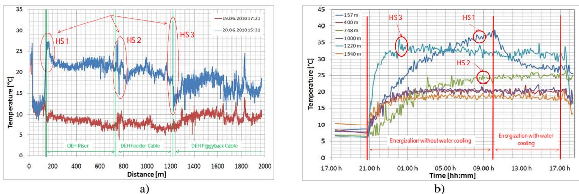
Figure 3. a) Temperature measured before (red) and during DEH Cable System Energization. Three hot spots (HS) are identified, and b) Temperature evolutions of the three HS and neighboring points before and during DEH energization.
