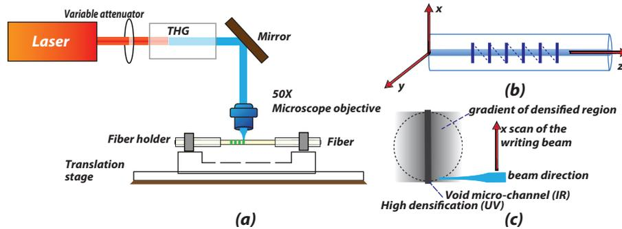
Figure 1. (a) Experimental setup for FBG inscription (b) schematic of top view LbL FBG inscription (c) transversal schematic view of the induced modification in the core (circle) and surrounded cladding area.
