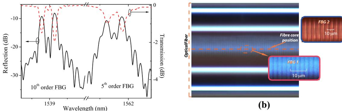
Figure 2. (a) Reflection and transmission spectra for 5<sup>th</sup> and 10<sup>th</sup> order 6 mm LbL FBG written with 2 µJ UV femtosecond beam. (b). Microscope image of the 5<sup>th</sup> order LbL FBG. Insets: close-up for 5<sup>th</sup> order FBG1 and 10<sup>th</sup> order FBG2.
