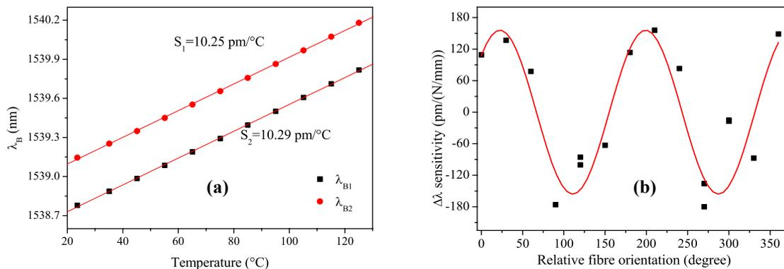
Figure 4. (a) Temperature and (b) transversal load of the 10<sup>th</sup> order LbL FBG.
