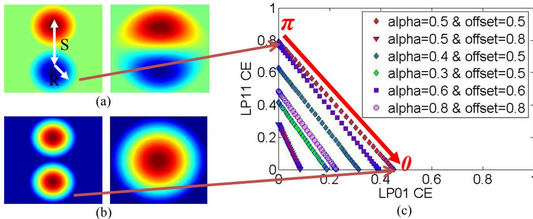
Figure 2. Push-pull solution for exciting (a) LP11 and (b) LP01 mode; (c) coupling efficiency for LP01 and LP11 modes with different alpha, offset and phase difference of two spots.
