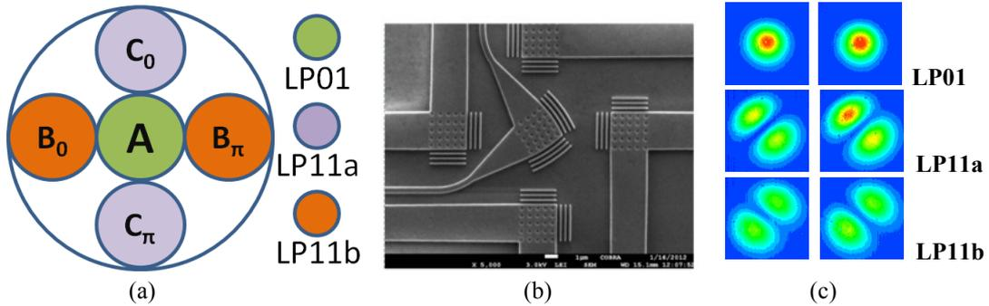
Figure 3. (a) A structure with 5 spots to serve for a FMF with 3 spatial modes; (b) the realization of this structure with a SOI integrated solution (A SEM image of the structure) and (c) Excited 3 spatial mode profiles with two polarizations.
