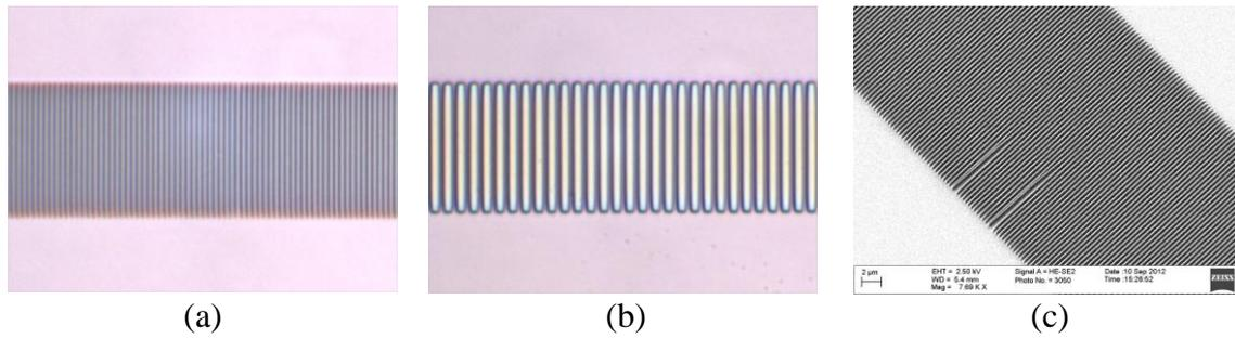
**Fig 1.** Strip-loaded, corrugated silicon nitride channel waveguide structures on a co-doped, planar monoclinic double tungstate layer with a period of a)  $\sim 0.5 \mu\text{m}$ , b)  $1.18 \mu\text{m}$ . c) Scanning electron microscope image of a corrugated channel with a period of  $\sim 500 \text{ nm}$ .
