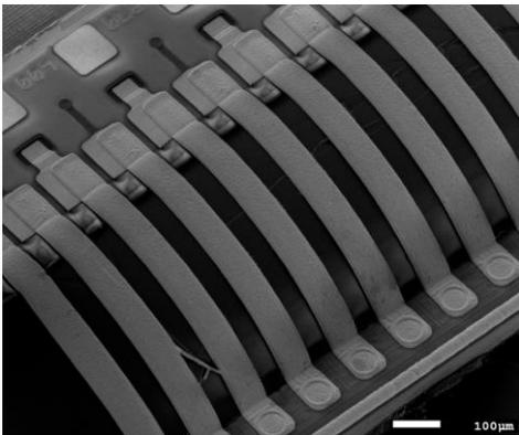
Fig. 1: (b) 3D stacking transmitter module
