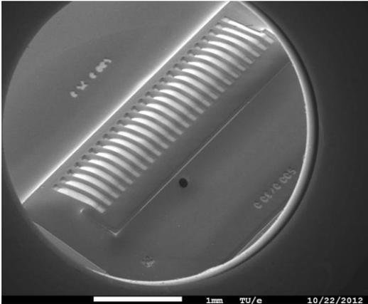
Fig. 3 (c) SEM image of the lithography between photodiode array and CMOS IC
