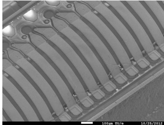
Fig. 3 (d) SEM image of the electrical path between PDs and CMOS driver IC
