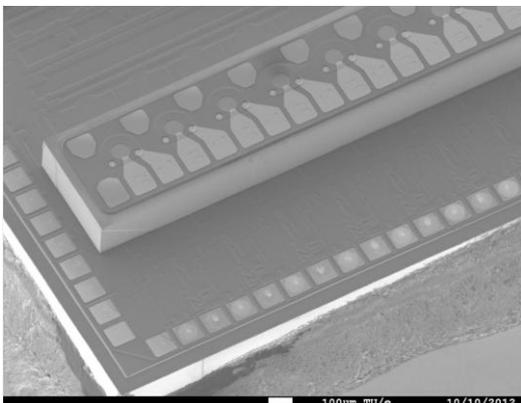
Fig. 3 (a) SEM image of photodiode array bonding on the TIA/LA CMOS IC
