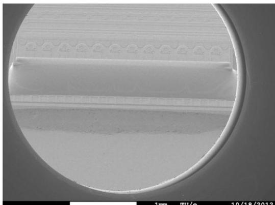
Fig. 3 (b) SEM image of photodiode array bonding on the TIA/LA CMOS IC
