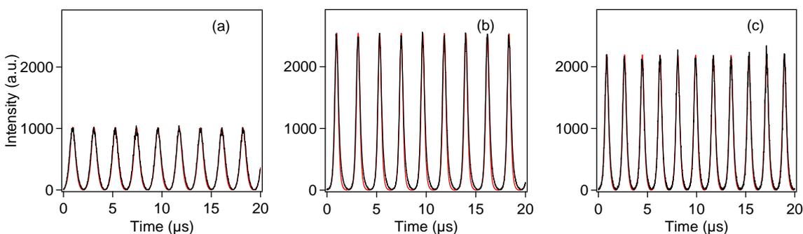
Fig. 2: Typical result of GA fit: the experimental pulse train (in black) and the calculated pulse train (in red) for three values of the pump power: (a) 2.86 W, (b) 3.7 W, and (c) 4.9 W.
