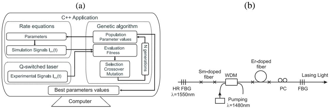
Fig. 1: (a) Diagram of the C++ application, including GA and the rate equations solving. (b) Self-Q-switched Er-doped fiber laser.
