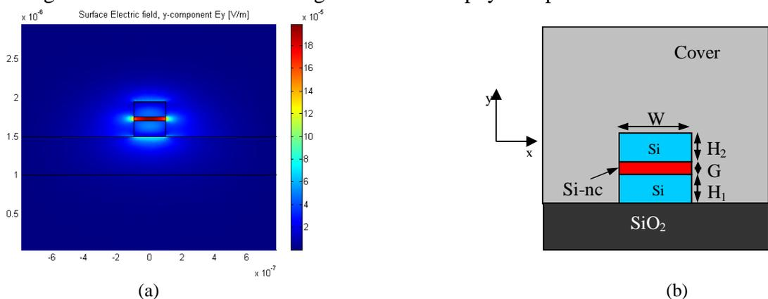
Fig. 1. (a) Cross section of SOI slot waveguide based on Si-nc; (b) 2D distribution of  $E_y$  component.
