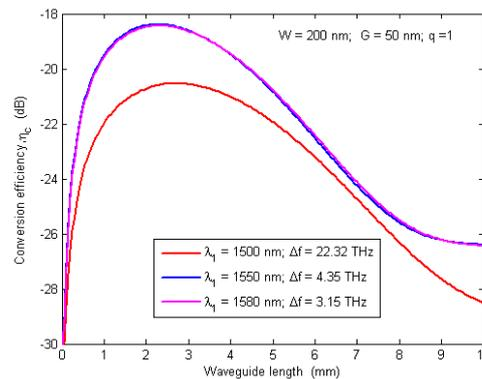
Fig. 5. Conversion efficiency versus the waveguide length.
