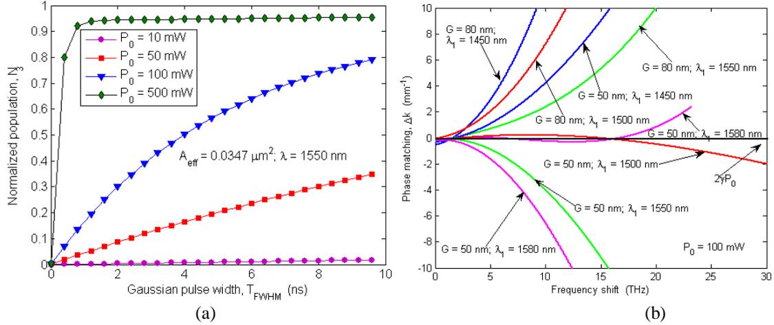
Fig. 3. (a) Normalized population  $N_3$  versus Gaussian pulse width for different values of peak power for various pump wavelengths and  $G$ ; (b) Phase matching  $\Delta k$  versus frequency shift.
