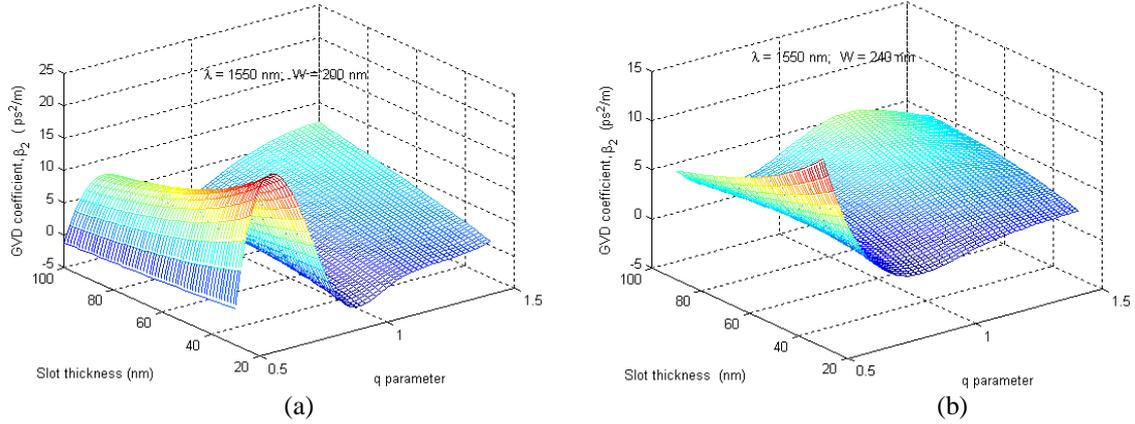
Fig. 2. GVD coefficient versus slot thickness  $G$  and  $q$  parameter: (a)  $W=200$  nm; (b) 240 nm.
