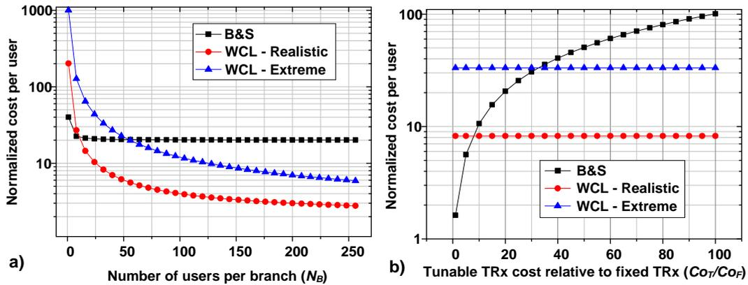
Fig. 3. Cost comparison between WCL-Access and conventional long-reach Broadcast-and-Select, cost is normalized to conventional PON TRx ( $Co_F$ ), a) cost per user as a function of number of users per branch, b) cost per user as a function of
