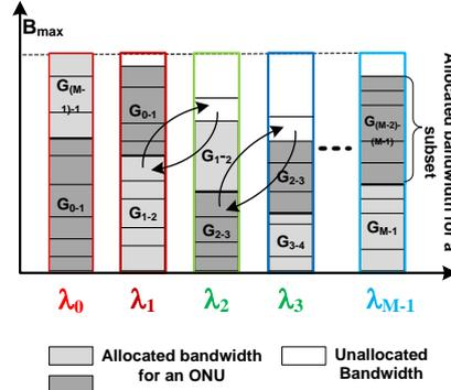
Fig. 2. Concept of bandwidth rearrangement where unallocated bandwidths are shifted toward a hot spot
