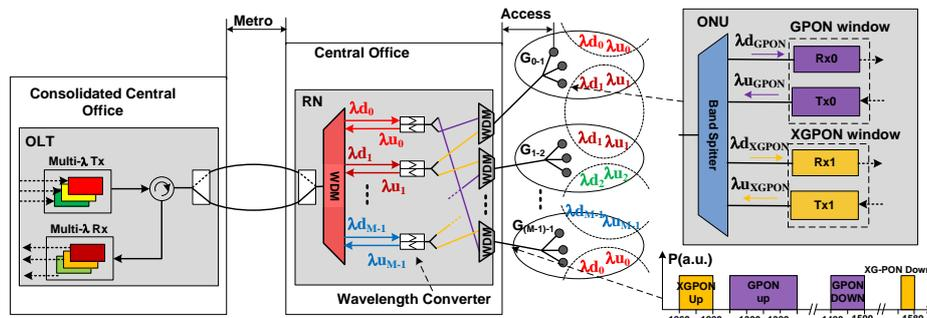
Fig. 1. Schematic representation of wavelength-converted long-reach architecture to support central office consolidation and direct migration for current PON deployments
