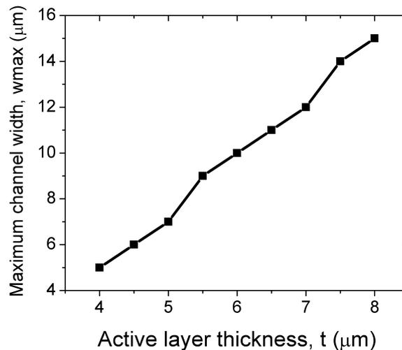
Figure 2: Maximum single-mode channel width,  $w_{\text{max}}$  as a function of waveguide thickness.
