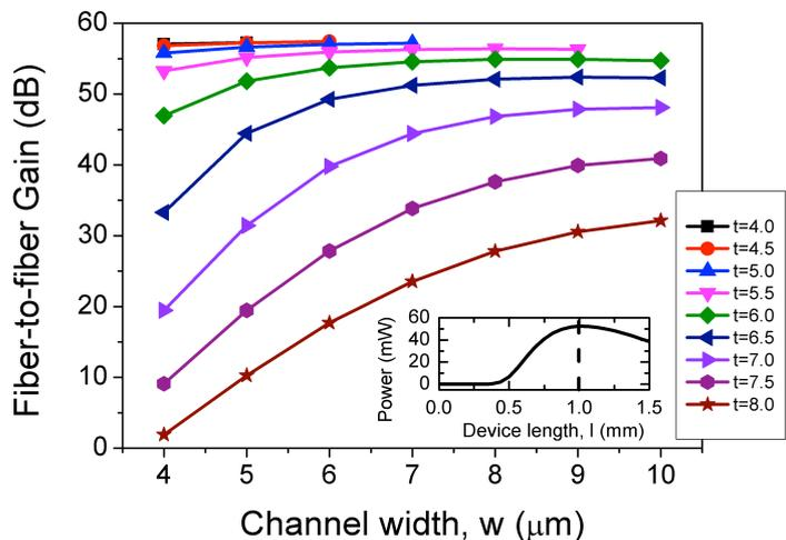
Figure 4: Simulated fiber-to-fiber gain for single-mode waveguide amplifier. Inset shows the evolution of the signal powers to the propagation distance for amplifier with  $w = 4.0$  and  $t = 4.0$
