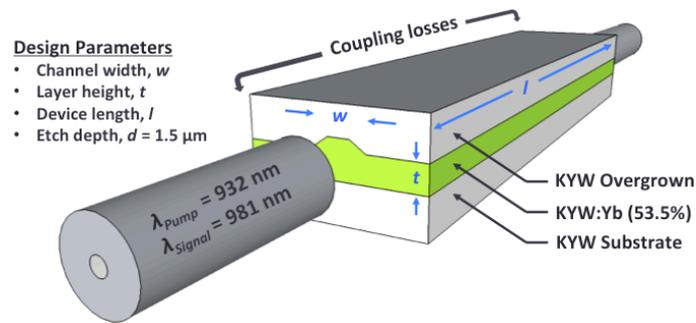
Figure 1: Schematic of the structural design of the channel waveguide amplifier.
