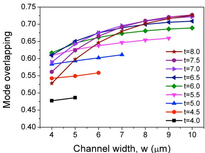
Figure 3: Overlap integral between the modal fields of the fiber and amplifier waveguide. The data for  $w$  exceeding  $w_{max}$  (i.e. those supporting multi-modes) is not shown in the figure.
