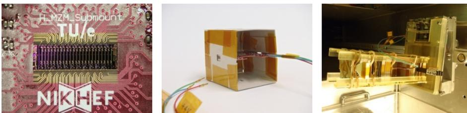
Fig. 2: (L to R) Modulator bar glued on the pedestal and bonded. Sub-mount PCB housed in a  $5 \times 5 \times 5$  cm<sup>3</sup> box for irradiation. Sub-mount PCB in the card-board box – loaded in the shuttle for irradiation.
