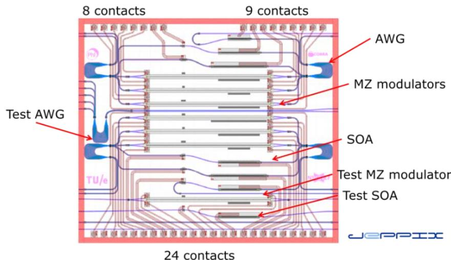
Fig. 4: ASPIC designed in the TU/e COBRA generic integration platform.
