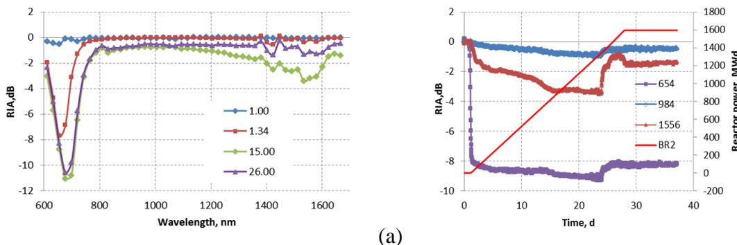
Fig. 5 RIA spectral evolution for fiber SMPS1000-125Al. The insets indicate (a) - times after the start of the experiment, (b) – wavelengths.
