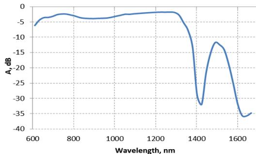
Fig. 6 Initial transmission spectrum of SMPS1000-125Al.
