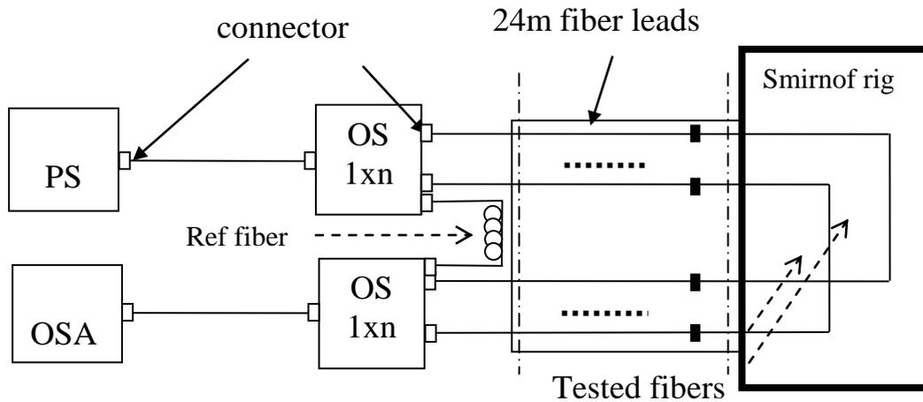
Fig.1 Schematics of the experimental set-up. PS – broad-band photonic source; OSA – Anritsu optical spectrum analyser, OS – optical switch.
