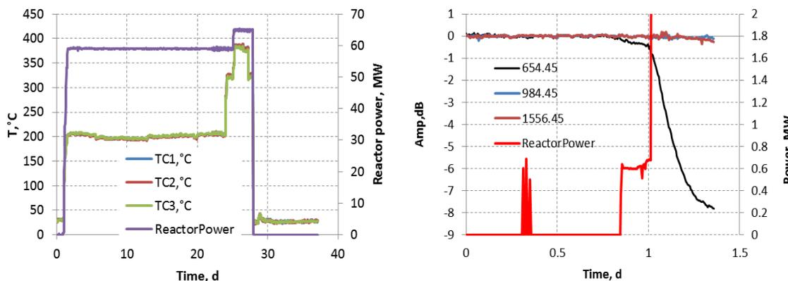
Fig.3 Variation of the temperature of the fibres and the reactor power during the experiment.
