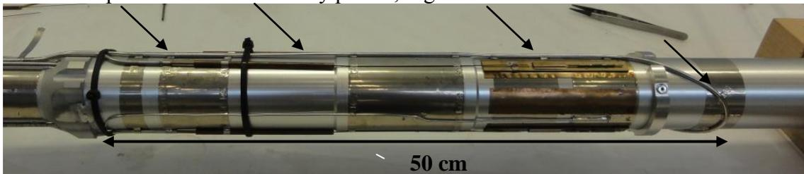
Fig.2 Part of the Smirnof rig placed inside the reactor core. The arrows indicate the tube with the fibres.
