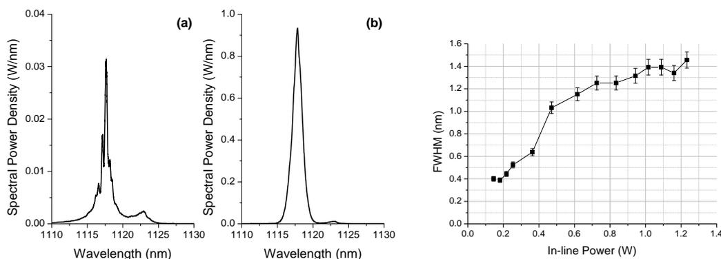
Fig. 2. Random DFB fiber laser spectrum generated in 500 m long nitrogen doped fiber near (a) and high above (b) the threshold. (c) Spectral width dependence on the generated power.
