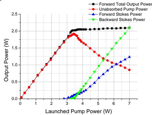
Fig. 1. Generated and pump power of the N-doped random DFB fiber laser.
