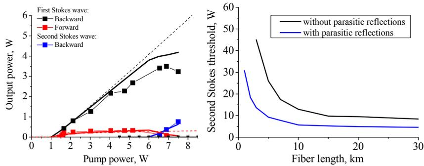
Fig. 1. (a) First Stokes (forward – red, backward - black) and Second Stokes (backward - blue) output powers for the random DFB laser based on 10.7 km TrueWave fiber: experimental data (boxes), numerical calculation without (dash) and with (solid) parasitic reflection. (b) Calculated generation threshold of second Stokes wave with (blue) and without (black) parasitic reflections of  $4 \cdot 10^{-5}$  at the fiber ends.
