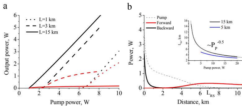
Fig. 2. (a) The forward and backward output powers for different fiber lengths (red – forward waves, black – backward waves). (b) The typical longitudinal power distribution of the pump wave and generated forward and backward wave. Pump power is 4 W. Calculations are made for TrueWave fiber and lasing at 1.2  $\mu\text{m}$ . Inset:  $L_{RS}$  dependence on pump power for different fiber lengths.
