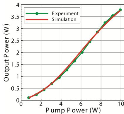
Fig.2. Total output power versus pump power in experiment and simulation
