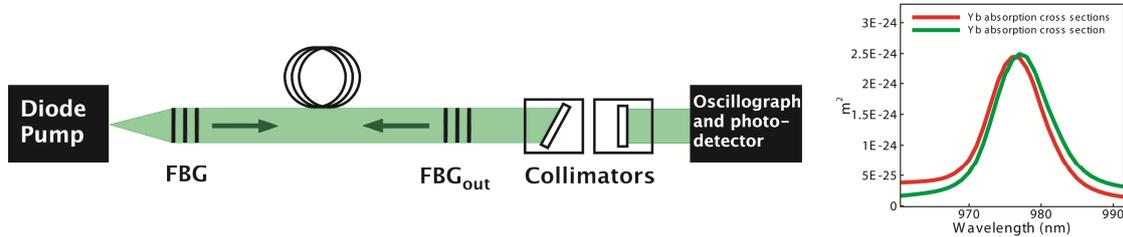
Fig. 1 (Left) Experimental setup. (Right) Ytterbium absorption and emission cross sections.
