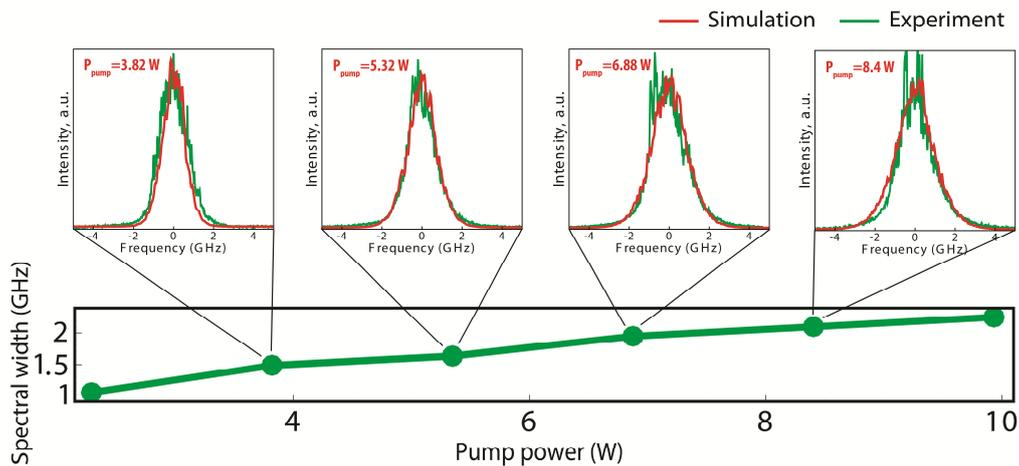
Fig. 3: (Bottom row) Output spectra width as a function of pumping power. (Upper row) Output spectra as a function of pumping power in experiment and simulation.
