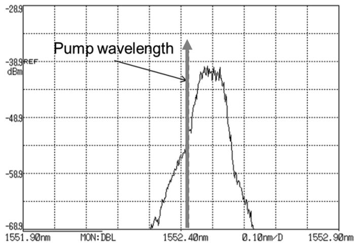
Fig.3 Optical spectra above Brillouin threshold at port A (a)
