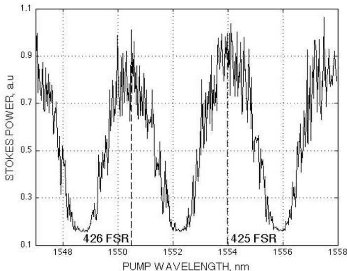
Fig.2. Stokes power at port A versus pump wavelength.
