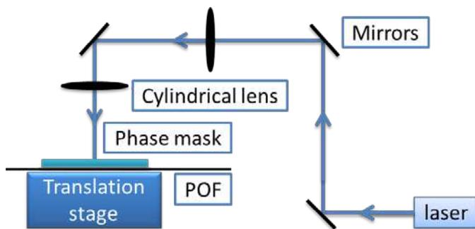
Figure 1: Sketch of the experimental set-up used for grating inscription in POF.
