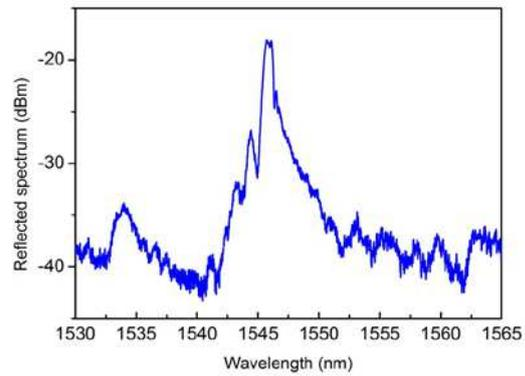
Figure 5: FBG reflected spectrum after 2.5h drying
