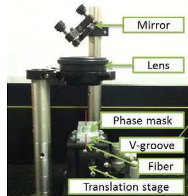
Figure 2: Real opto-mechanical devices in the experiment.
