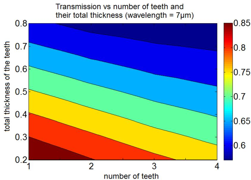
Figure 2: Transmission versus the number and total thickness of the teeth. The total thickness is the ratio of the sum of the teeth thicknesses over the total grating thickness.
