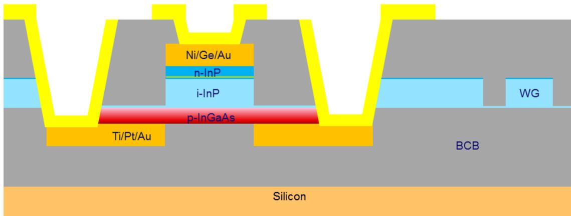
Fig. 1. Cross-section of the UTC-PD (not to scale)
